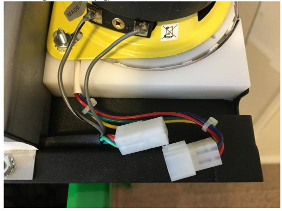
4. Insert existing male plug into female coupler of supplied splitter/power extension, plug the free male plug of the splitter into the female connector leading to the existing speaker LEDs, then tuck everything into cavity above
