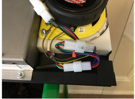
5. Run the RGB+ power extension through the existing wire loom down into the main cabinet. Be sure to leave plenty of slack for lowering the speaker panel in the future.
