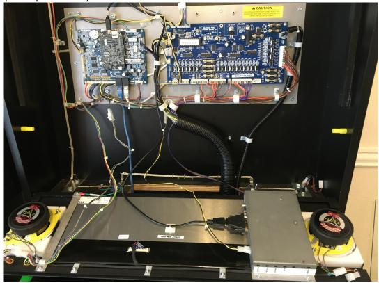
3. De-couple the RGB+ connector to the right speaker (you may need to use a flathead screwdriver to pry the clips on opposite sides enough to release the plug).
